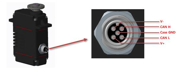
3-2 Cable and Pin Assign (SG Series CAN Cable Type)
